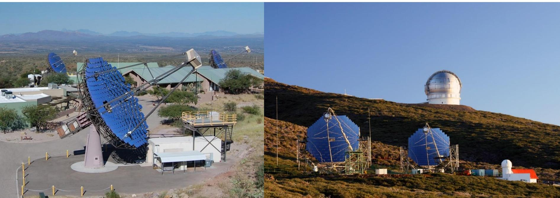
**Fig.) Imaging Atmospheric Cherenkov Telescopes (IAC**Ts
