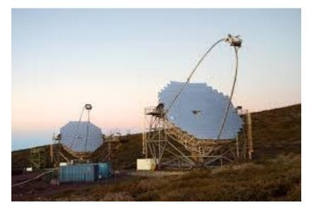
Fig.) Examples of Imaging **Atmospheric Cherenkov telescopes (IACTs).**
